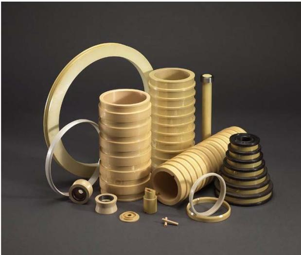
ZIRCOX ceramic components have distinct advantages over carbides & coated steels. Extreme hardness, excellent surface finish and chemical product inertness are all factors that reduce the level of impact on the die and improve wire quality. All our ceramic cones, capstans, pulleys and draw rings in our Zircox series have these advantages and suitable for ferrous & non-ferrous wire drawing applications.
